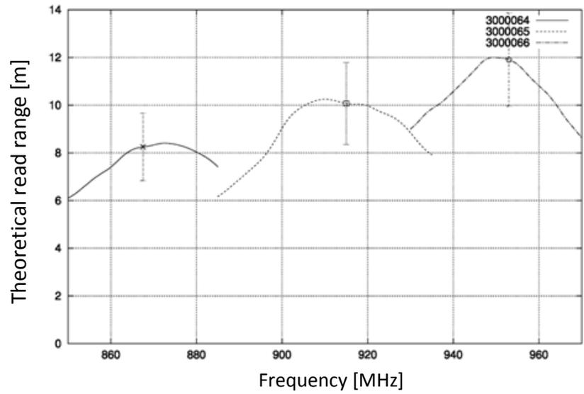
\* Read ranges are theoretical values that are calculated for non-reflective environment, in where antennas with optimum directivity are used with maximum allowed operating power according to ETSI EN 302 208 (2W ERP). Variation of 3σ from test batch marked in the picture. Note, tag performance in other frequency bands is not marked in the picture; tag will remain functional but the performance is low.
